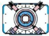
TEVATRON B = 4 \text{ T} Bore : 76 mm
