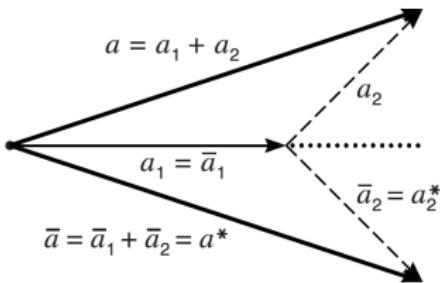
Case for 2 interfering amplitudes  $a_1$  and  $a_2$  with only weak phases.
