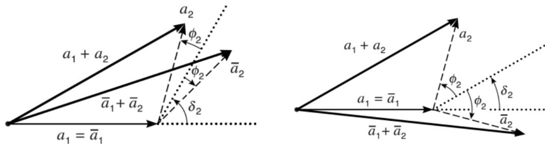
Case for 2 interfering amplitudes  $a_1$  and  $a_2$  with weak ( $\phi$ ) and strong ( $\delta$ ) phases.
