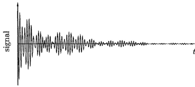
Fig. 3.12 A simulated free induction decay signal. The oscillations die away with time due to spin-spin relaxation ( T_2 processes). The data show an interference pattern which results from three inequivalent nuclei, each of which experiences a slightly different magnetic field because of their different sites within a crystal.
