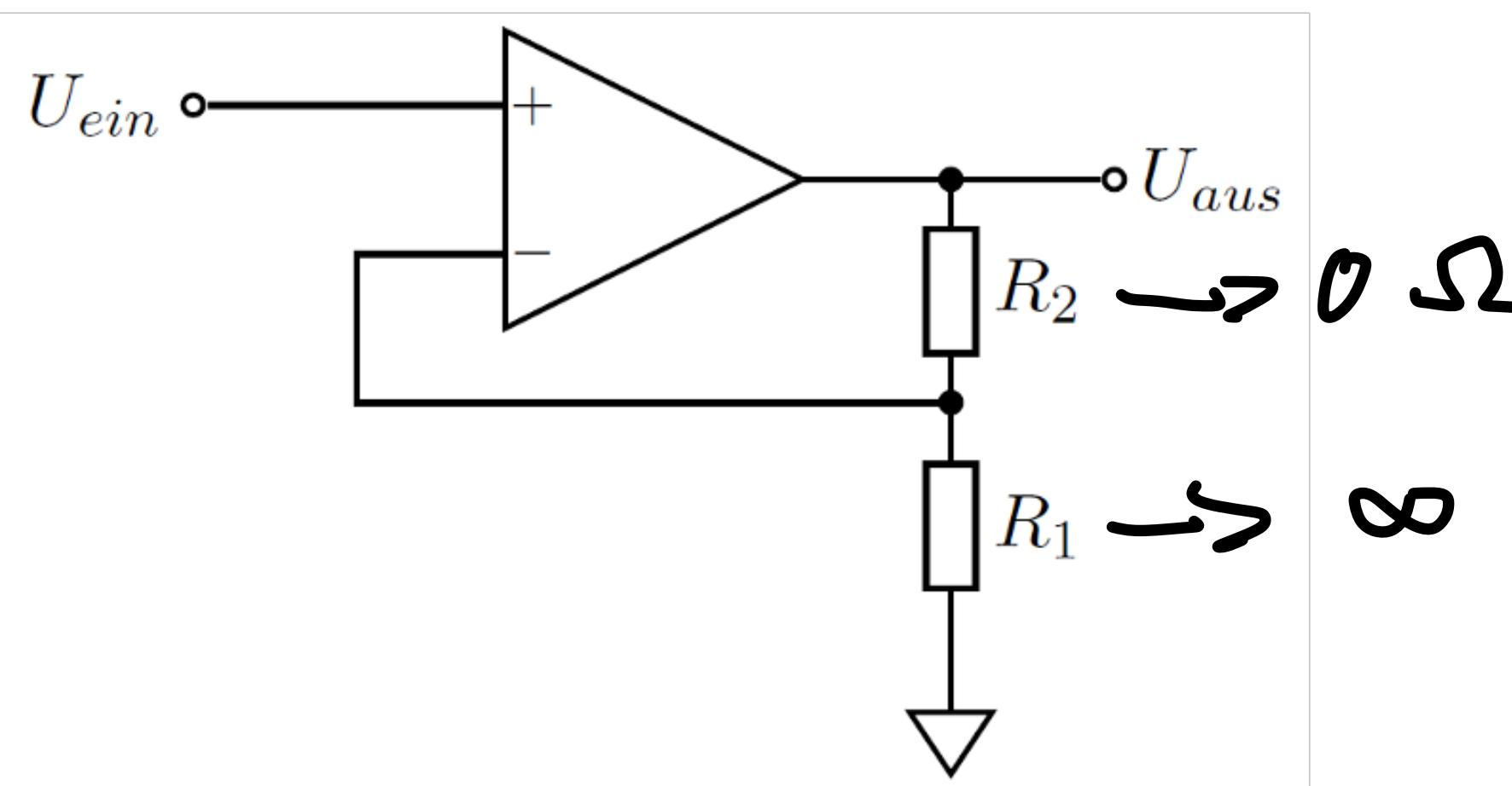
But: Output current can be high (small output impedance of OpAmp) without putting a load on the input source.
