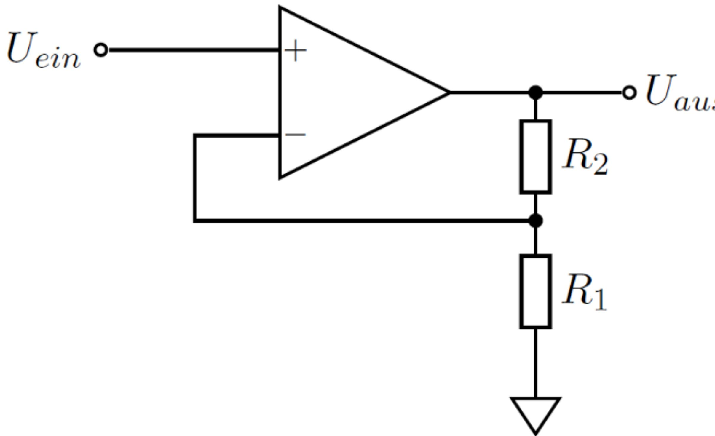
Input signal into the non-inverting input
