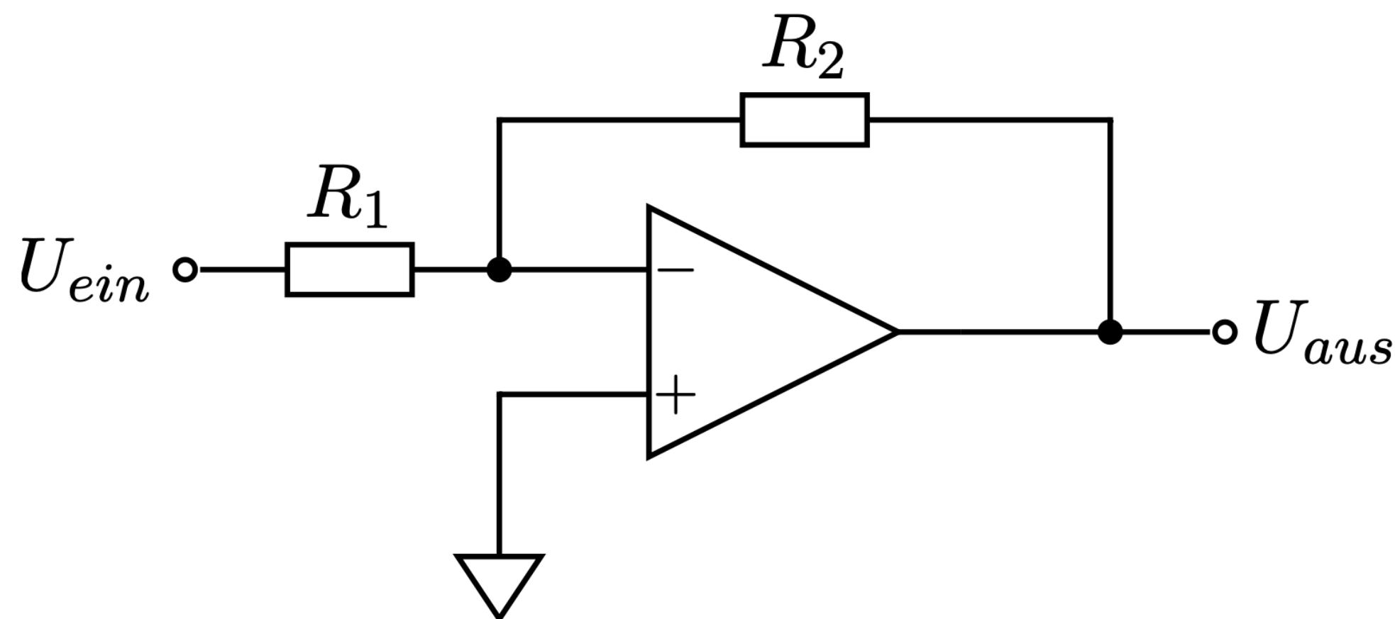
$$K_F = -\frac{R_2}{R_1 + R_2}$$
