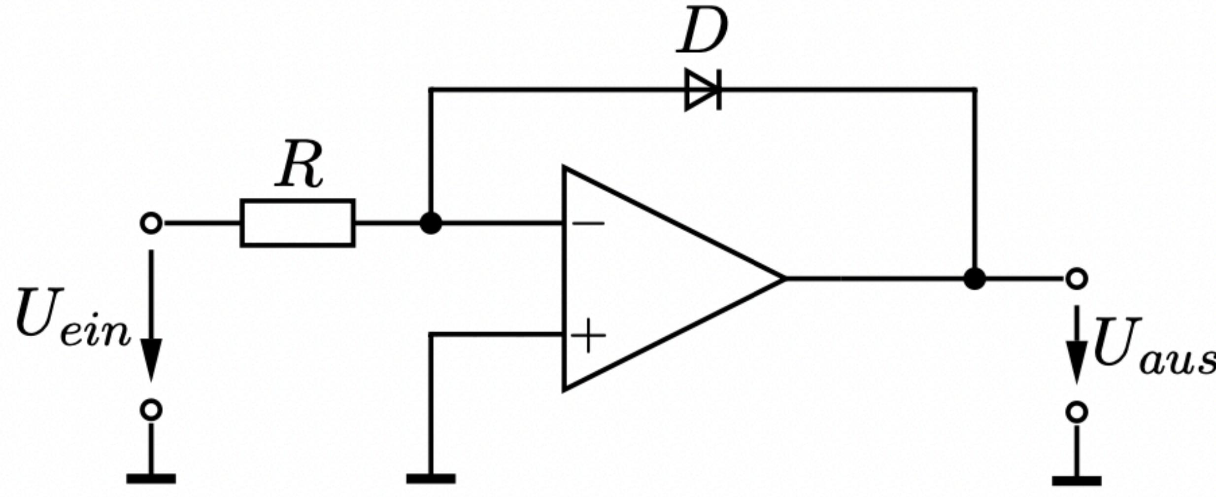
Using the exponential IV curve of a forward-biased diode:
