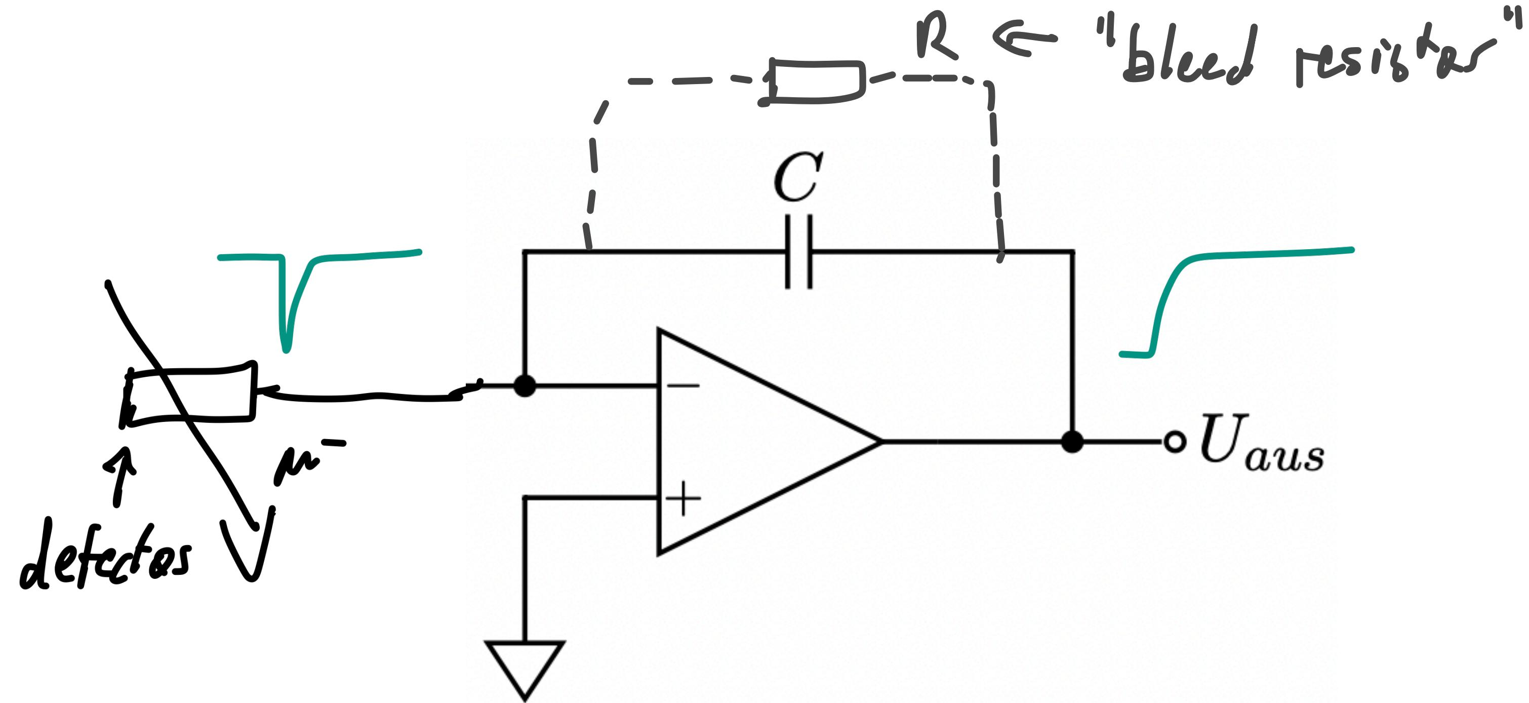
Important application: charge-sensitive pre-amplifier for particle detectors.
