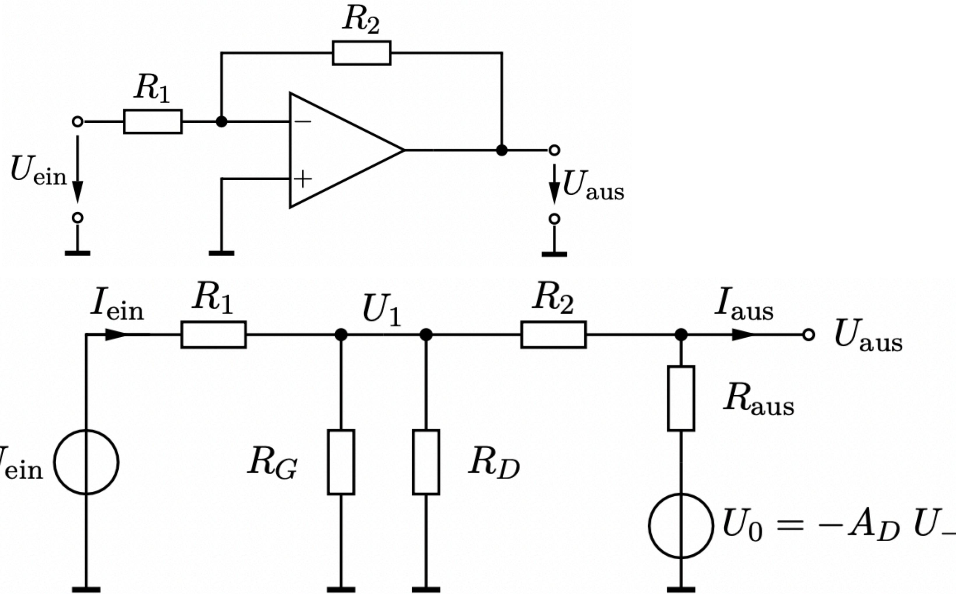
$U_- = U_1$  Voltage on inverting input
