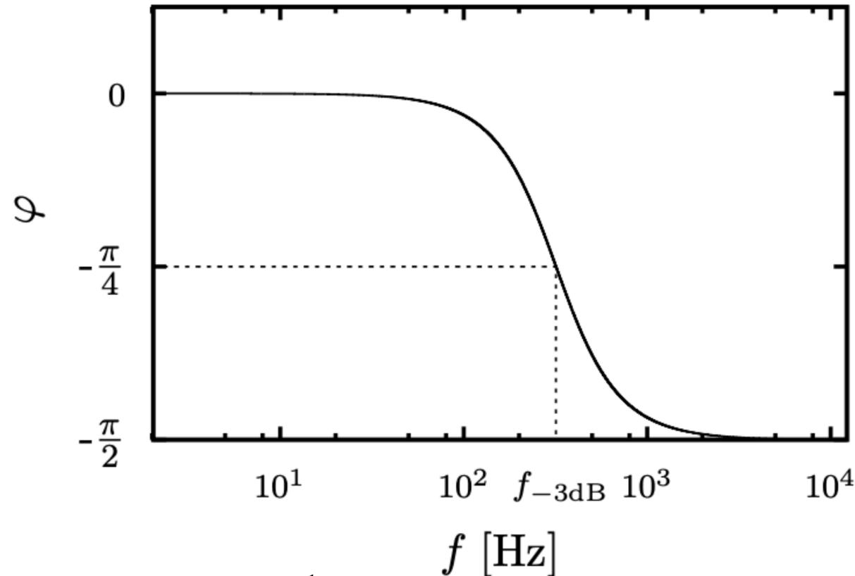
$$Z = \frac{1}{\sqrt{1 + (\omega RC)^2}} \quad \tan \varphi = -\omega RC$$
