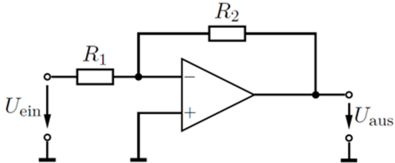
$$I_{\text{ein}} = U_{\text{ein}}/R_1 \text{ (since } U_- = 0\text{)}$$
