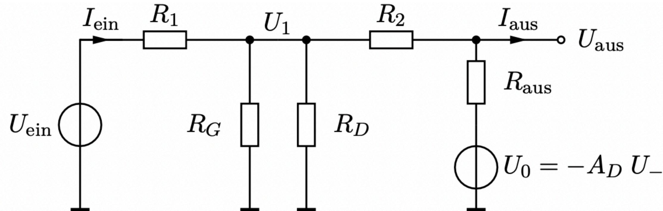
$U_- = U_1$  Voltage on inverting input
