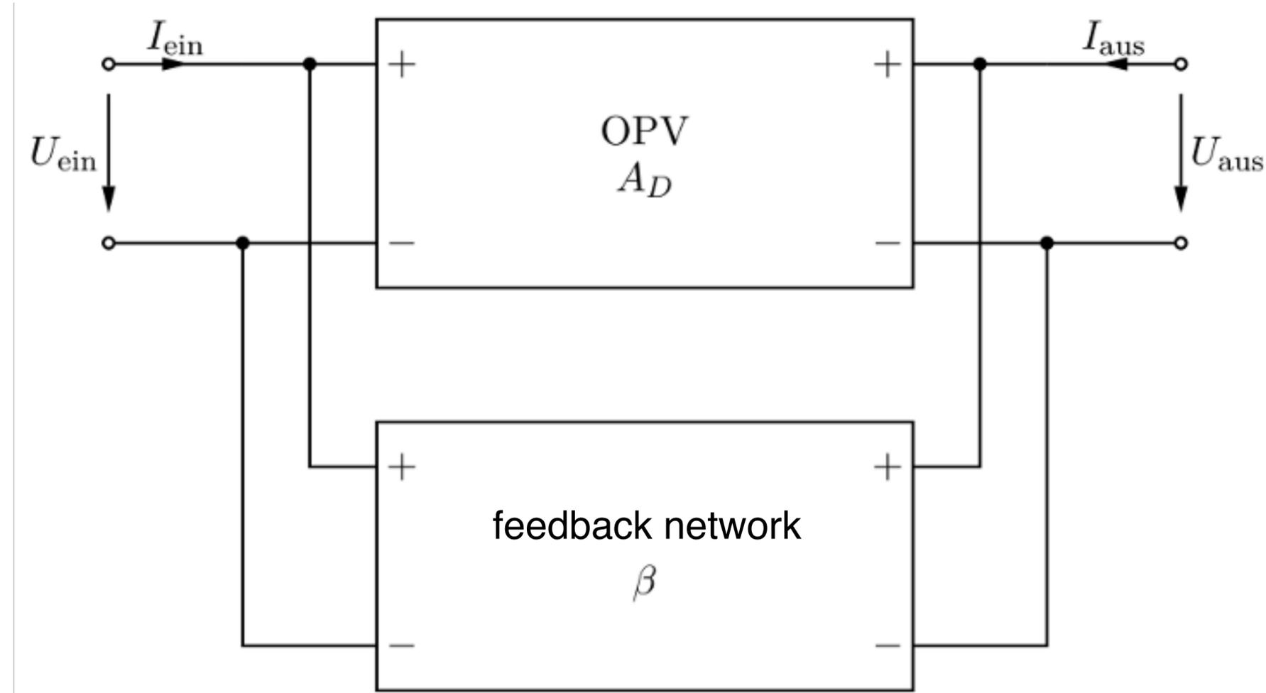
OpAmp parallel (“shunt”) on input and output of the feedback network: “shunt - shunt”
