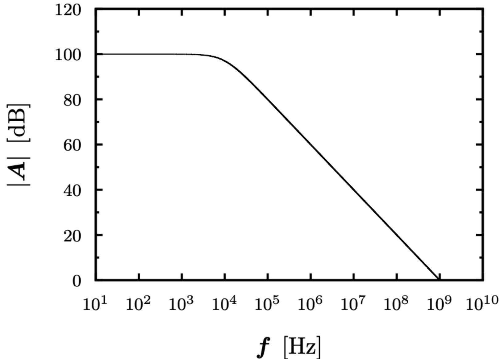
Gain drops significantly beyond cutoff frequency ("Grenzfrequenz)  $f_g$
