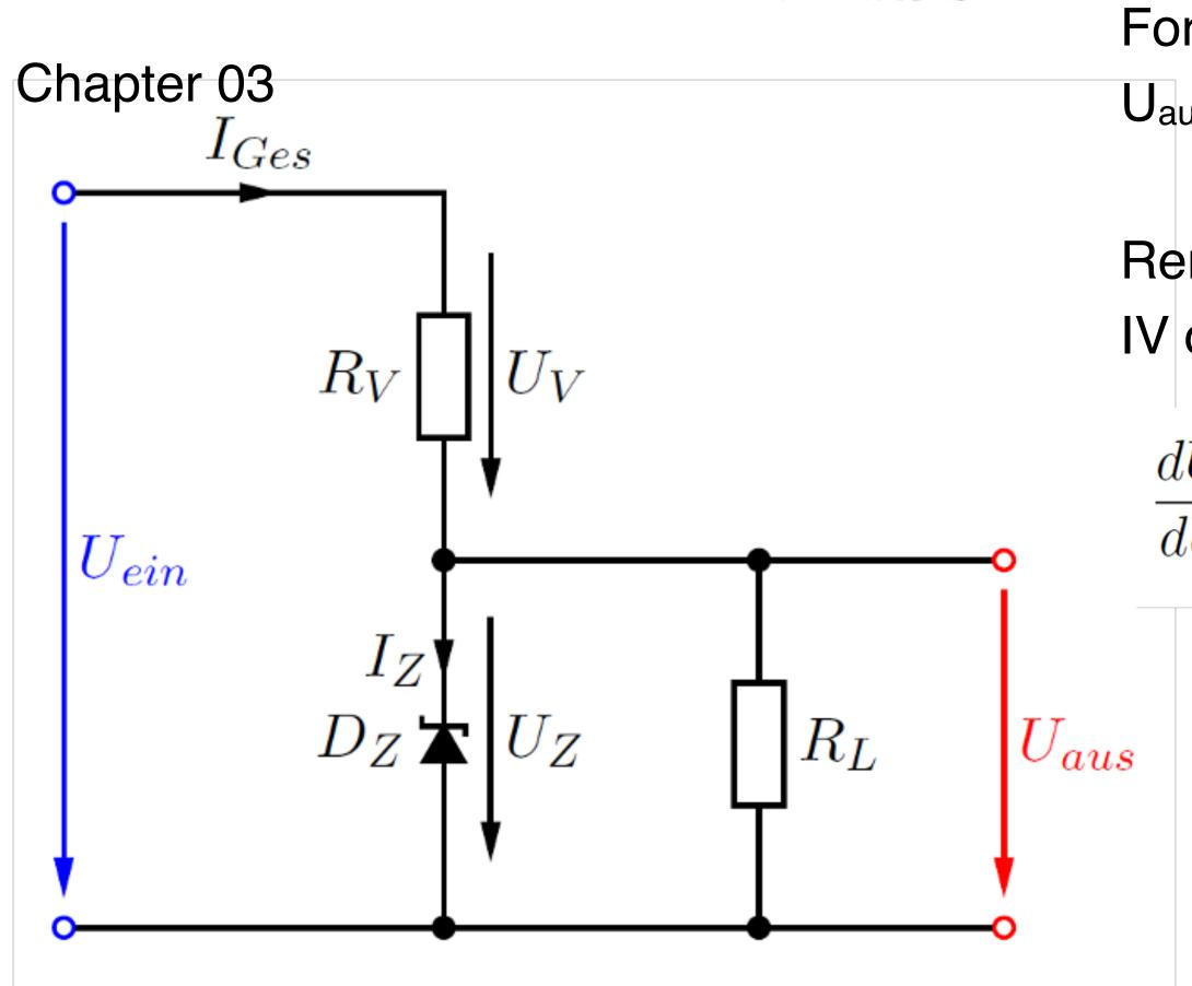
Simple, but hits limits for high load currents. Strong temperature dependence due to diode.
