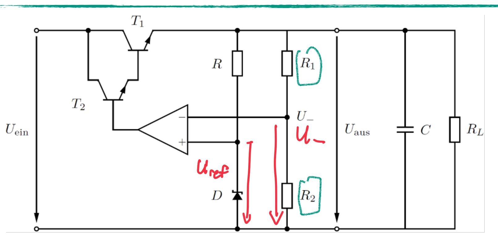
Darlington transistor T<sub>1</sub>, T<sub>2</sub>: Enables high load currents
