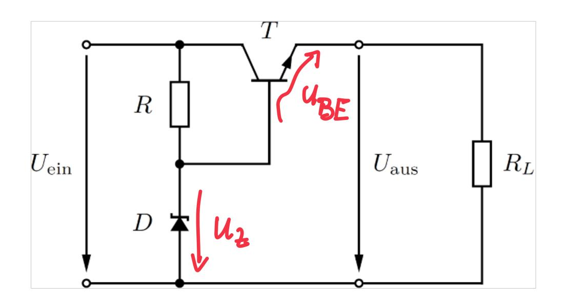
But:  $U_{BE}$  depends on current: not constant - typically between 0.5 V and 0.8 V  $U_{aus}$  only stable to within a few 100 mV!
