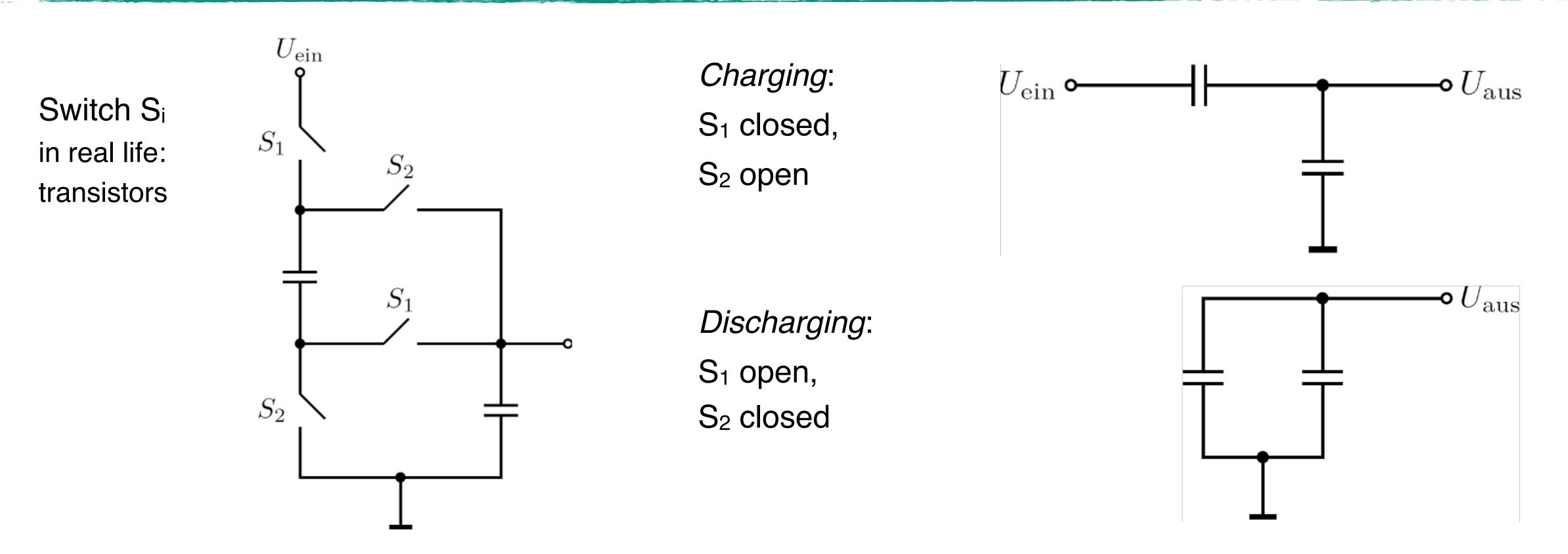
high switching frequency to achieve low fluctuations in output voltage: typically kHz - MHz
