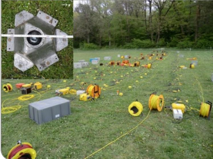
Area 31m x 27 m, 52 3-C Galpherin source locations ("UVW"), 896 3-C geophones (4.5 Hz, "XYZ"), 6 days, repetition of all source positions for each geophone patch
