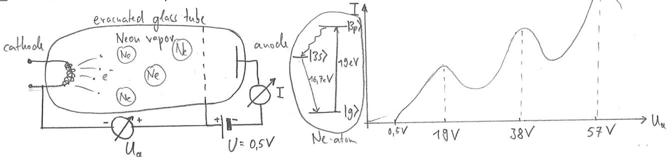
a) The energy of the emitted electrons increases with  $E_{pot} = e \cdot U_a$ . Every 19V in acceleration voltage they have accumulated enough potential  $\rightarrow$  kinetic energy to excite a Neon atom a further time by collision. At that point they might not have enough energy to reach the anode  $\rightarrow$  the anode current drops.
