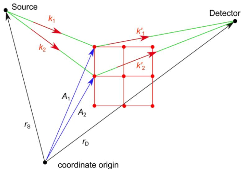
parallel beams can be used because the crystals are small and the distances in the x-ray diffractometer are large
