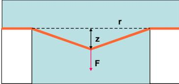
Restoring Force  $F_R$  in z-direction for a membrane deformed to a cone:
