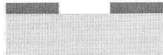
(c) Develop photoresist pattern
