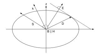
In an anisotropic medium the electric field vector and the displacement field are not parallel anymore:
