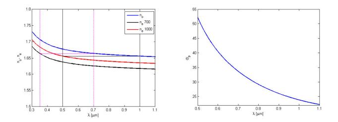
Dispersion diagram indicating the phase matching angle for  $\lambda = 700$ nm and  $\lambda = 1000$ nm and phase matching angle over wavelength
