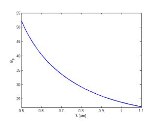
Dispersion diagram indicating the phase matching angle for  $\lambda = 700$ nm and  $\lambda = 1000$ nm and phase matching angle over wavelength
