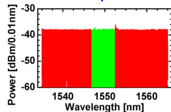
⇒ 325 carriers with 12.5 GHz spacing, linewidth < 10 kHz
