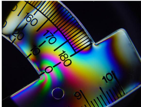
Visualization of the **elasto-optic effect**: The medium becomes birefringent under strain, leading to interference fringes in a polarized-light image.
