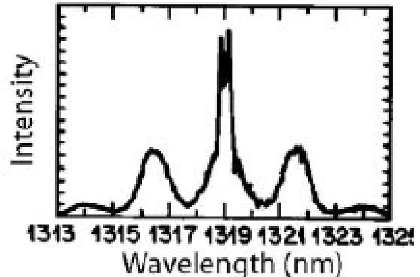
Sidebands at fiber output occurring as a consequence of modulation instability.
