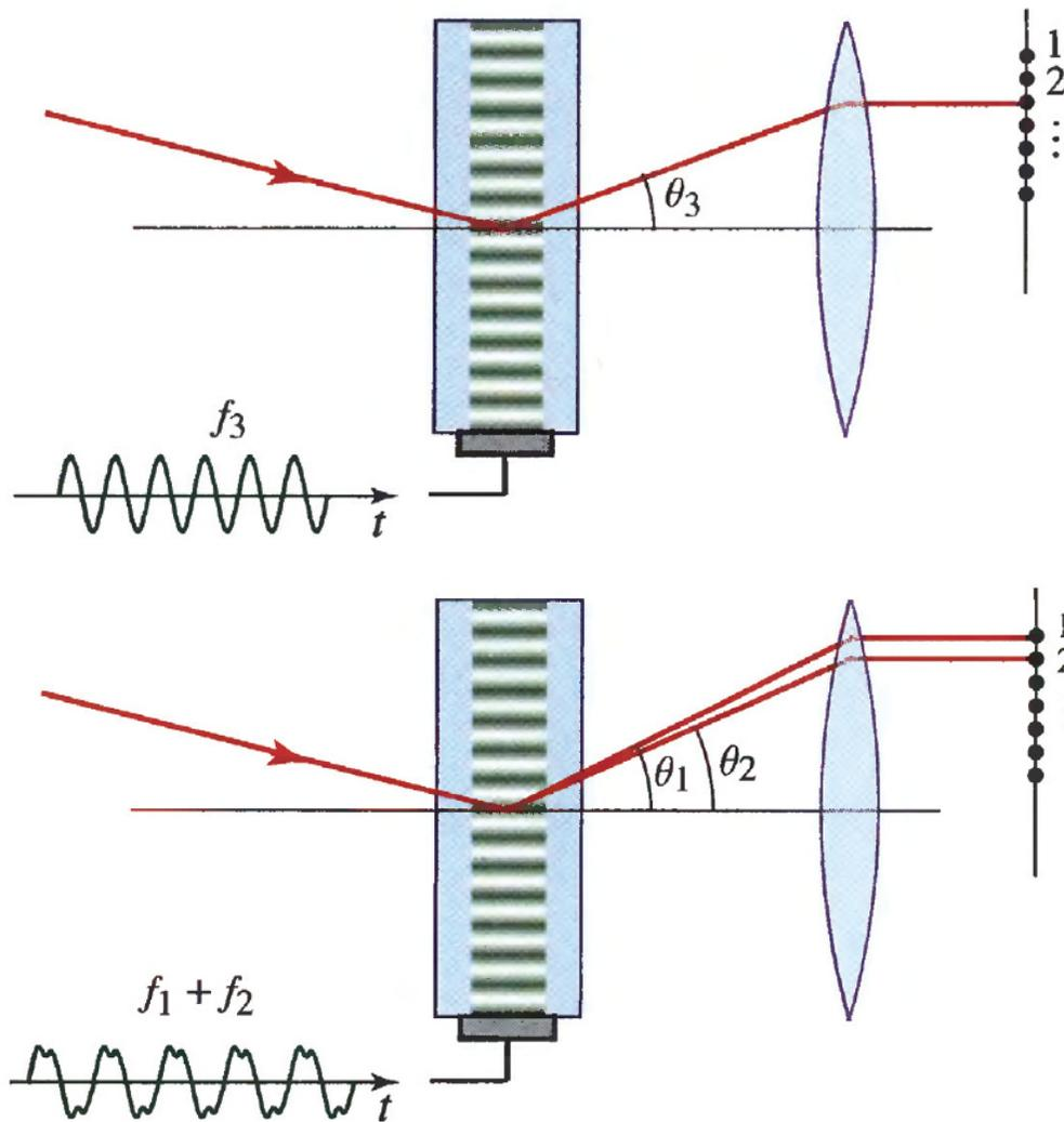
**Splitting** of incident optical beam by using acoustic drive signals that comprise various frequency components
