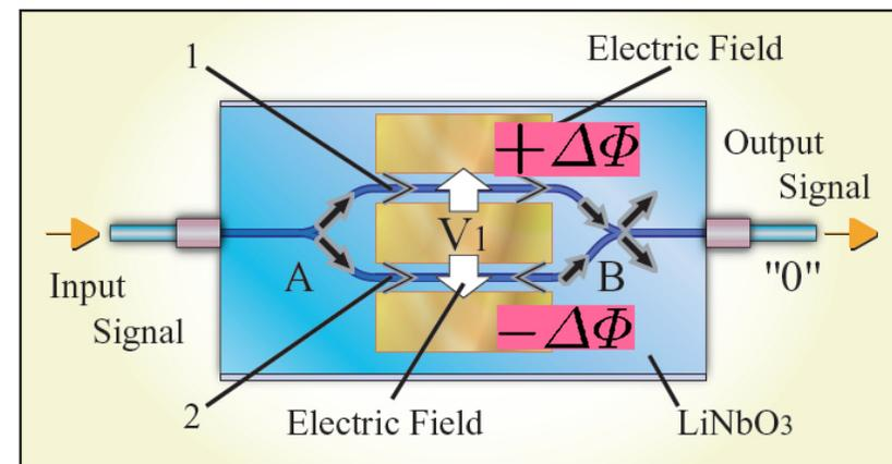
Here: Push-pull configuration, i.e., antisymmetric phase shifts in both arms of the interferometer (same magnitude, opposite sign)
