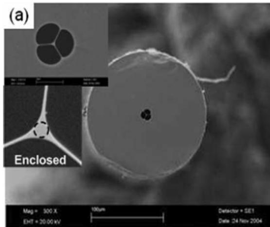
Supercontinuum generation in a highly nonlinear fiber with ultra-small mode field diameter
