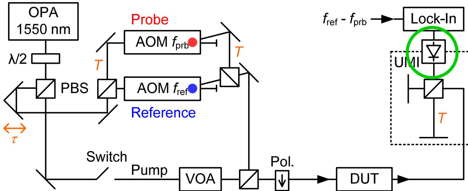
Beat signal at difference frequency at  $f_{\text{ref}} - f_{\text{prb}}$  detected by lock-in amplifier in amplitude and phase!
