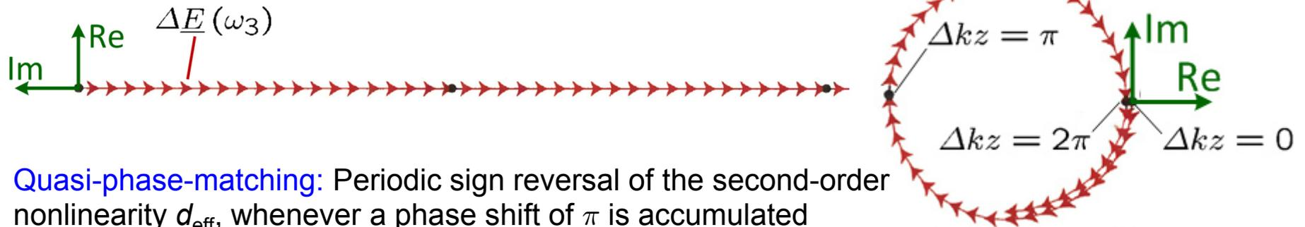
**Quasi-phase-matching:** Periodic sign reversal of the second-order nonlinearity  $d_{\text{eff}}$ , whenever a phase shift of  $\pi$  is accumulated
