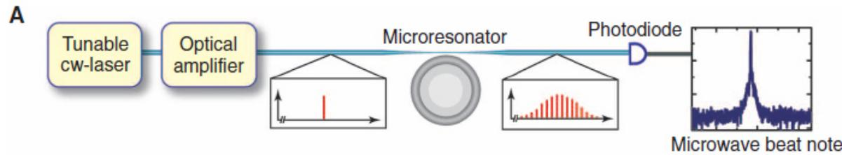
High-Q optical resonator “stores” sideband photons and enables generation of further sidebands by four-wave mixing
