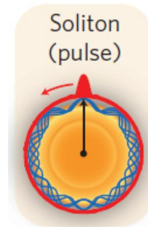
Superposition of all resonator modes leads to formation of a cavity soliton
