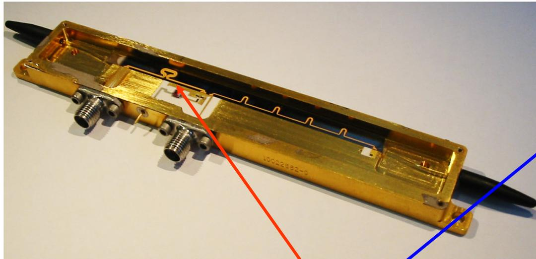
State-of-the-art  $\text{LiNbO}_3$  amplitude modulator
