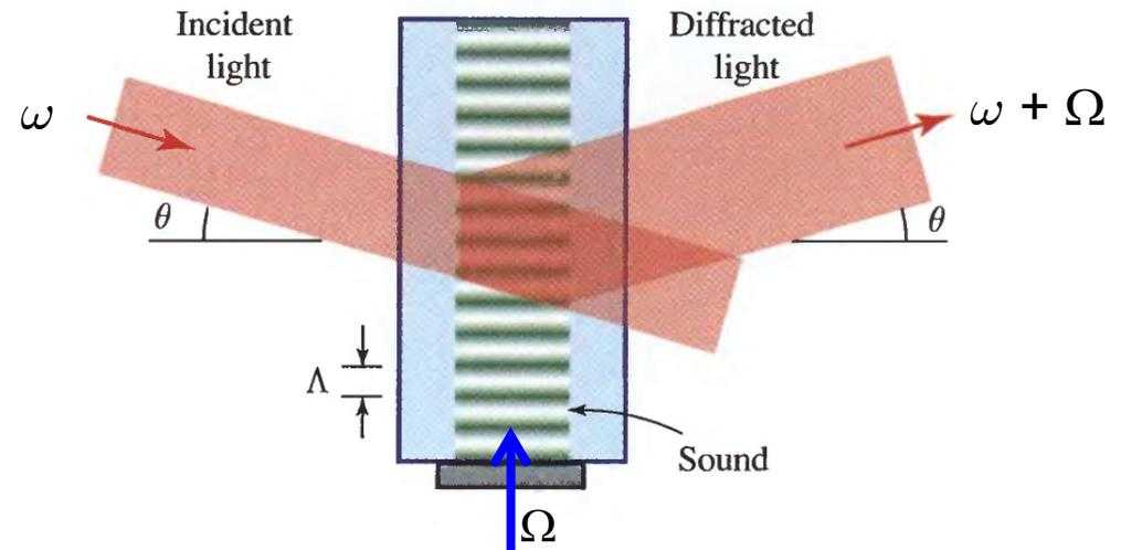
**Application example:** Optical vibrometry
