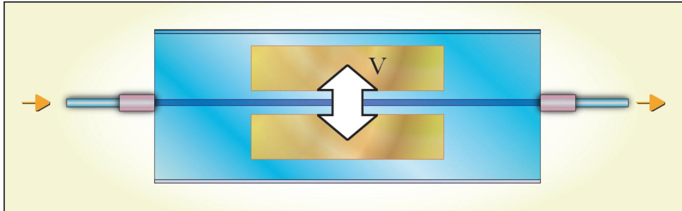
Turning a phase modulator into an amplitude modulator: Mach-Zehnder Modulator (MZM)
