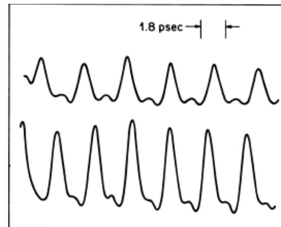
“Seeded” modulation instability using two different probe wavelengths
