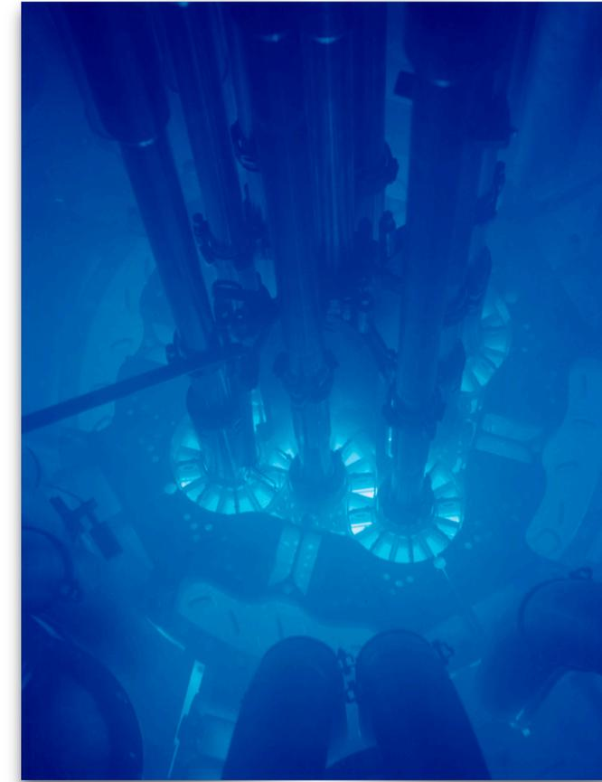
Cerenkov radiation in cooling water of the Idaho nuclear test reactor
