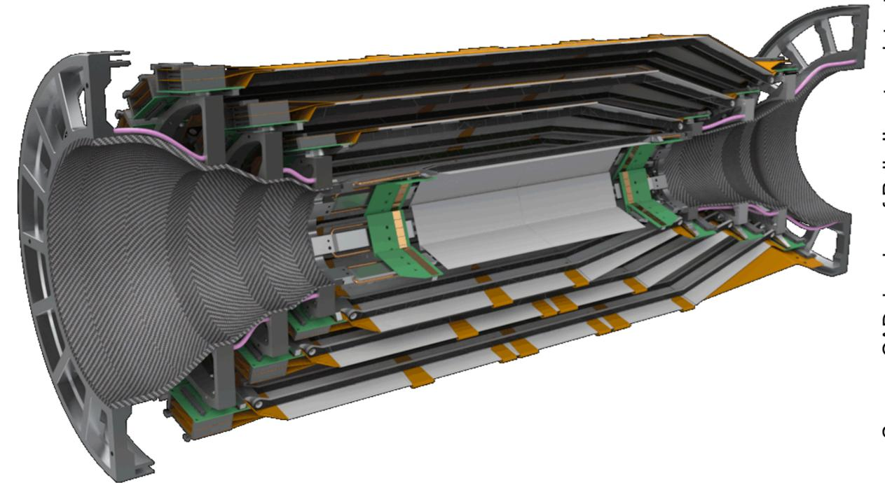
Source: CAD drawing of Belle II vertex detector
