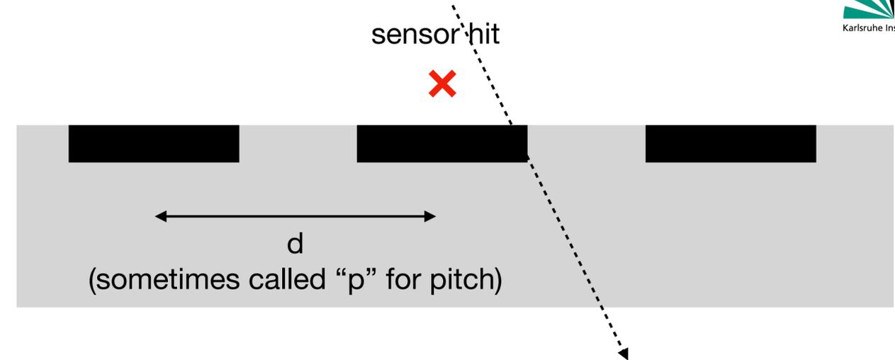
Digital readout: additional information about charge or time → Resolution better than  $\sigma < d/\sqrt{12}$
