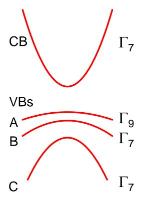
Band structure including labeling of CB and VBs according to their irreducible representations at the  $\Gamma$  point
