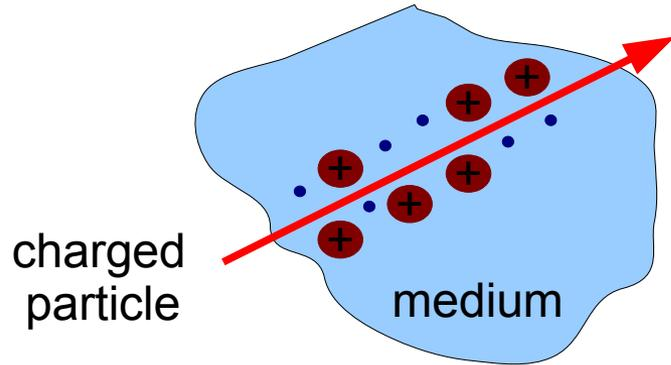
average number of ion-electron pairs is proportional to particle energy
