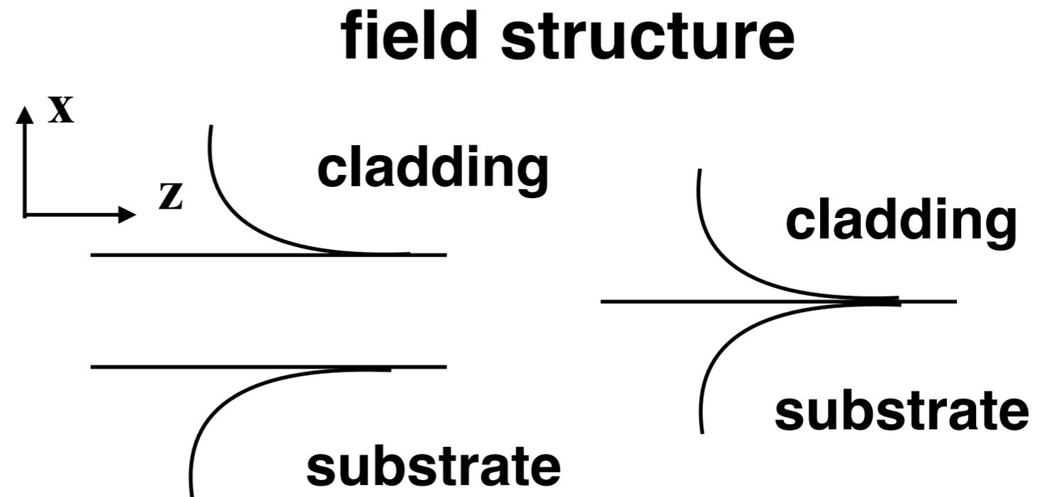
**note the modified principle propagation direction**
