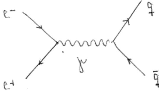
Figure 6.5: Feynman diagram for the process  $e^+ + e^- \rightarrow q + \bar{q}$ .
