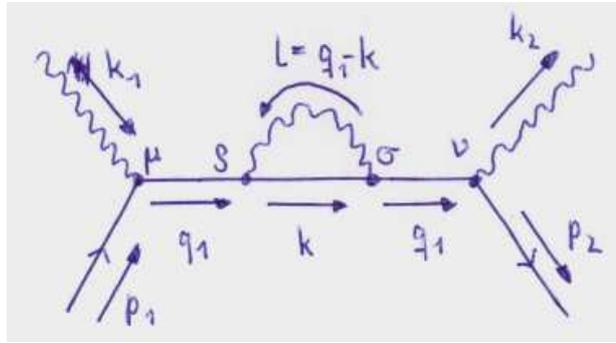
Figure 5.7: Diagram contributing to Compton scattering at order  $e^4$ . (Remark: The arrow for the momentum  $l$  has to be in the opposite direction.)
