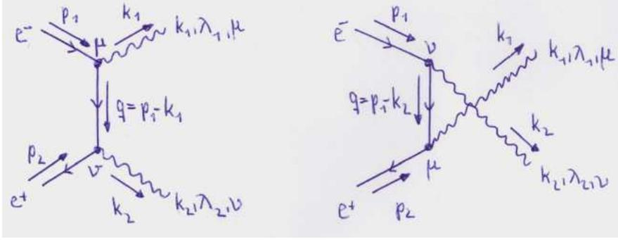
Figure 5.5: Diagrams contributing to pair annihilation. (Remark: In the second diagram the momentum of the fermion propagator between the two photon vertices has to read  $q' = p_1 - k_2$ .)
