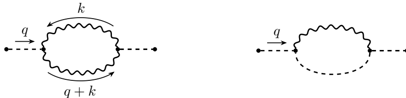
Figure 2: Non-abelian corrections to the Coulomb gluon propagator with two(left) and one(right) transverse gluons.
