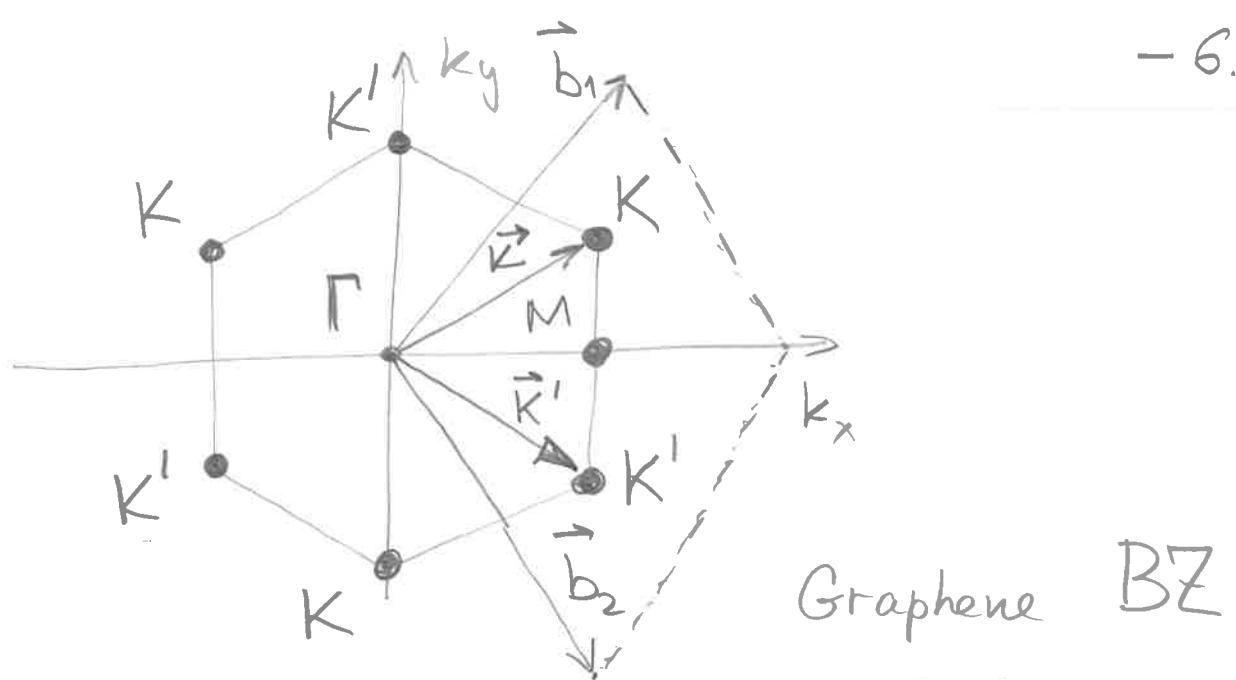
$$\vec{K} = \frac{2\pi}{3a} \begin{pmatrix} 1 \\ 1/\sqrt{3} \end{pmatrix}, \quad \vec{K}' = \frac{2\pi}{3a} \begin{pmatrix} 1 \\ -1/\sqrt{3} \end{pmatrix}$$
