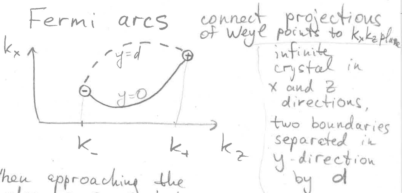
When approaching the nodes, surface states penetrate deeper and deeper to the bulk; at the circles, they are completely mixed with bulk states: the Fermi arcs on opposite boundaries are connected at Weyl points through the bulk.
