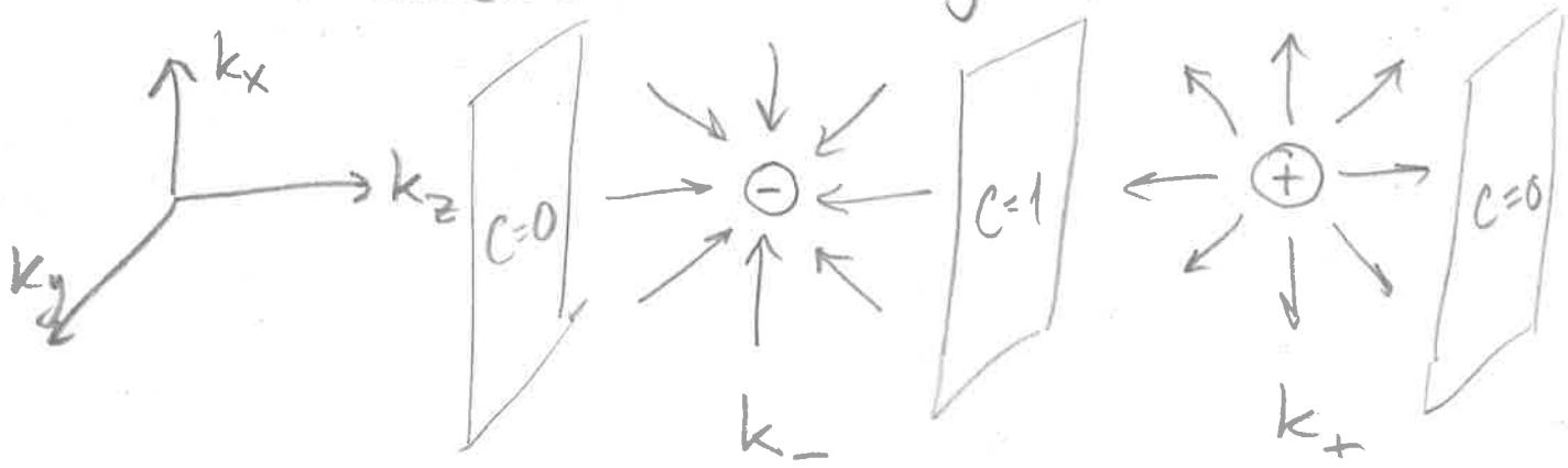
Treat  $k_z$  as a parameter: for each slice of  $k_z$  there is a 2D band structure that depends on  $(k_x, k_y)$ . Except for  $k_z = k_{\pm}$ , there is a gap in 2D bands at Fermi energy.
