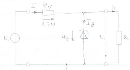
$$R_L = \frac{U_a}{I_L} = 66\Omega \Rightarrow E24 : 68\Omega \Rightarrow I_L = 48,5mA$$
