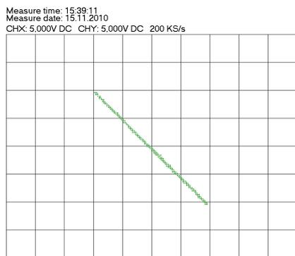
(c)  $f_1 = f_2 = 500\text{Hz}$  Phasenversatz  $\varphi = 0$
