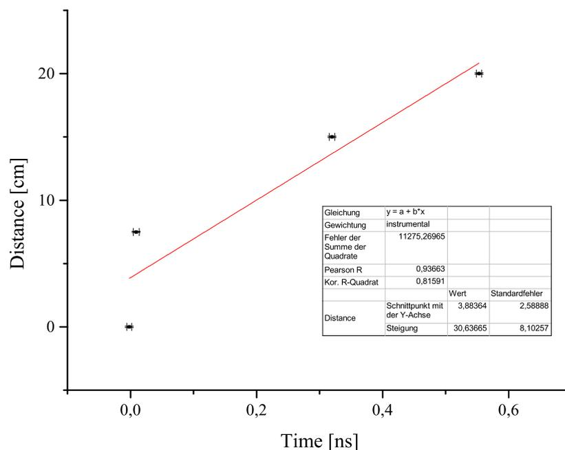
Figure 7: Linear fit for determining the speed of light.
