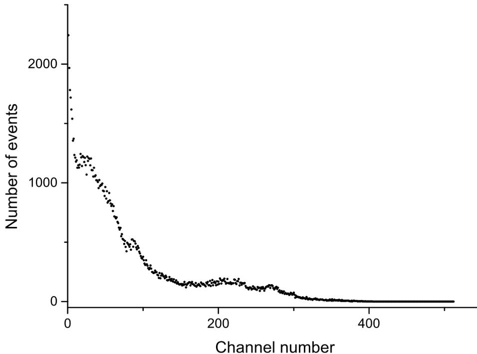
Figure 3: Full spectrum of  $^{22}\text{Na}$ .
