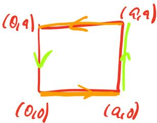
$$\oint_C d\vec{r} \cdot \vec{f}(\vec{r}) = \int_0^a dx (f_x(x,0) - f_x(x,a)) + \int_0^a dy (f_y(a,y) - f_y(0,y))$$
