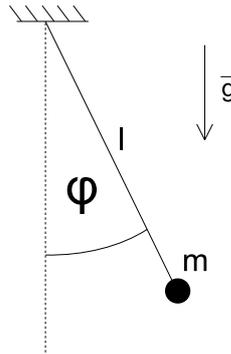
$$\mathcal{L} = \frac{ml^2}{2}\dot{\varphi}^2 - U(\varphi) = \frac{ml^2}{2}\dot{\varphi}^2 + (\cos \varphi - 1) mgl$$
