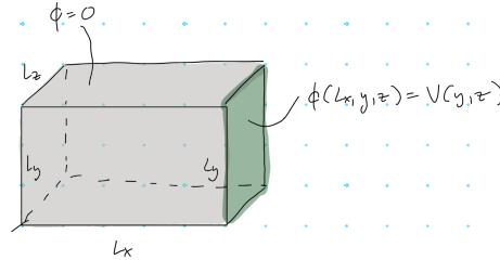
$$z: \phi(x, y, z) = \sum_{m, n=1}^{\infty} d_{mn} \sinh\left(\sqrt{\left(\frac{m\pi}{L_x}\right)^2 + \left(\frac{n\pi}{L_y}\right)^2} x\right) \sin\left(\frac{m\pi y}{L_y}\right) \sin\left(\frac{n\pi z}{L_z}\right) \quad (4)$$
