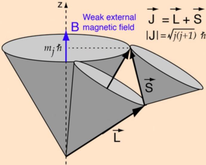
In the weak field case the vector model at left implies that the coupling of the orbital angular momentum  $L$  to the spin angular momentum  $S$  is stronger than their coupling to the external field. In this case where [spin-orbit coupling](#) is dominant, they can be visualized as combining to form a total angular momentum  $J$  which then precesses about the magnetic field direction.
