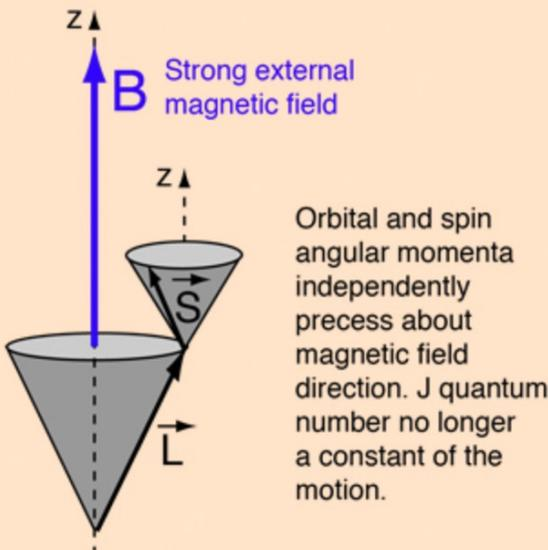
In the strong-field case,  $S$  and  $L$  couple more strongly to the external magnetic field than to each other, and can be visualized as independently precessing about the external field direction.
